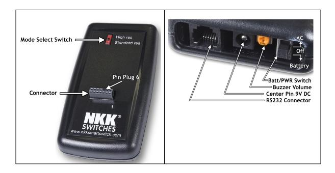
The **Mode Select Switch** has two settings; "High res" is for the High Resolution (64x32) switches/ displays and "Standard res" is for the Standard RGB switches/ displays.
